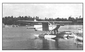
and whenever possible should have an L or T shaped configuration to provide approaches into the wind. The facing or apron around the dock should project deeply enough into the water to prevent chines and spray rails from catching - a common source of float damage. If the dock is located in an area of heavy pleasure boat or commercial water traffic. placing the dock between the boats and aircraft will lessen the hazards of wake damage.
